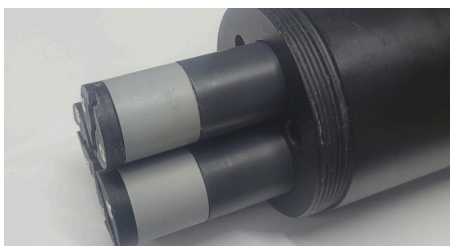
Figure 47 - 3 x selective ion sensors inside a multiparameter housing.
