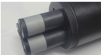
Figure 39 - 3 x selective ion sensors inside a multiparameter housing.
