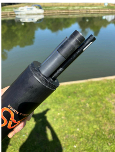
Figure 49 - a pH sensor inside a multiparameter housing.
