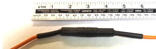
Figure 19 Sealed Connector with Heat Shrink Cover
