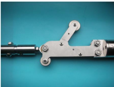
Figure 10 - Connection of a Spacer Bar to the Wheel Assembly
