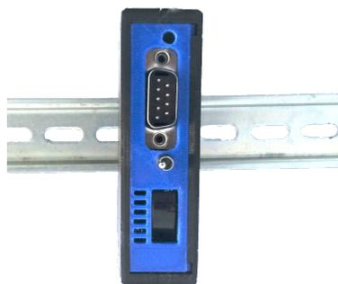
Figure-5 - VibWire-301 mounted on DIN Rail
